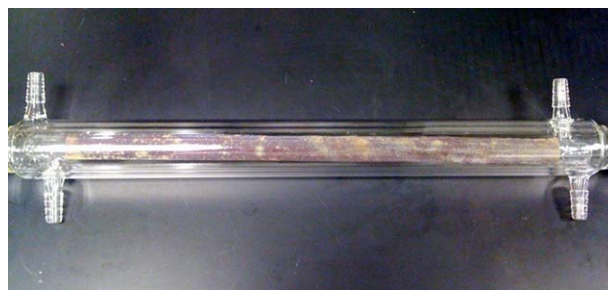
Figure 6. Layer crystallization apparatus used in the experiments.
